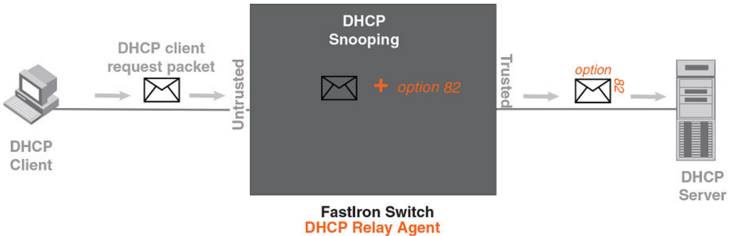
FIGURE 13 DHCP option 82 attributes added to the DHCP packet
